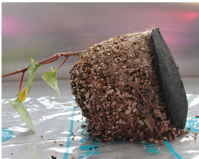
Figure 10: Japanese knotweed sample with no root growth either through or around the CuTex layer. Vigorous root growth can be seen in the vermiculite layer.
