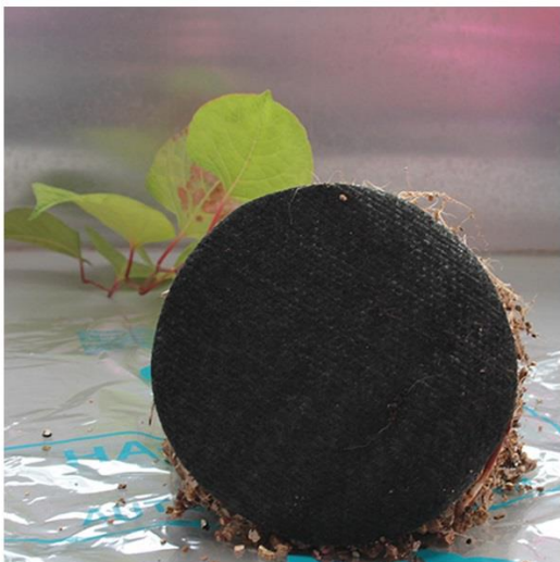
Figure 10: Japanese knotweed sample with no root growth either through or around the CuTex layer. Vigorous root growth can be seen in the vermiculite layer.
